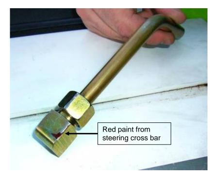
Figure 7. Red paint smear on the broken elbow connector
