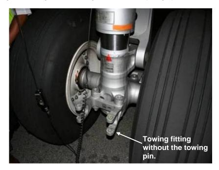
Figure 3. Nose gear towing fitting with the towing pin missing
