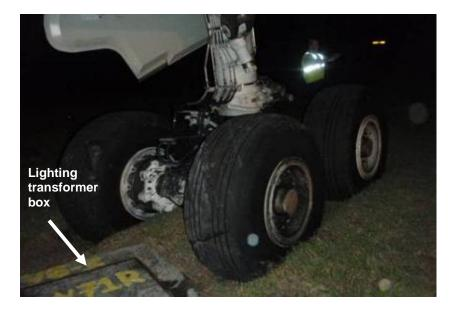
Figure 2. Right wing landing gear and the concrete airfield lighting transformer box
