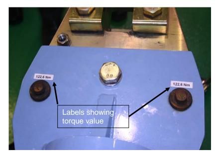
Figure 8. Labels on the tow bar showing the required torque value
