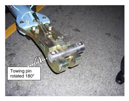
Figure 6. Tow bar clamp holding towing pin detached from towing fitting and rotated 180°
