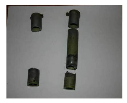
Figure 5. Sheared fuse pins of the towing fitting
