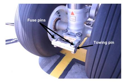
Figure 4. Nose gear towing fitting with fuse pins and towing pin in place
