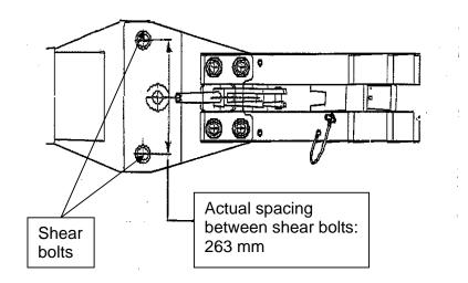
Figure 9. Spacing between the two shear bolts on tow bar
