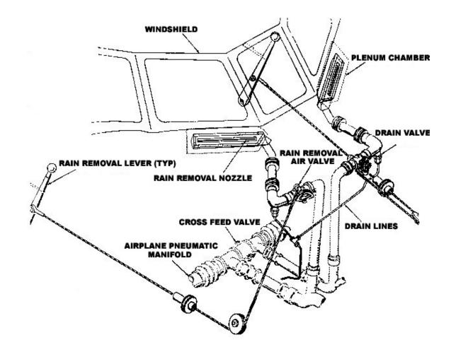
Figure 1. Windshield rain removal system
