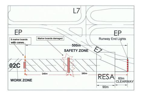
FIGURE 1 - Position of the first row and second row of marker boards
