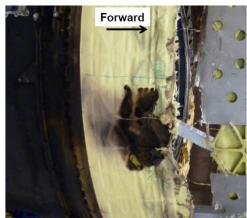
Figure 15: Burnt Kevlar at bottom of engine
