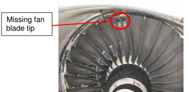
Figure 2: One fan blade had a missing tip section (front view)
