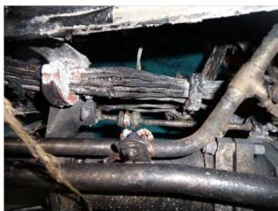
Figure 13: Fire damage to electrical harness near fuel flow transmitter
