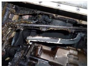
Figure 11: Fire damage to the AOHE
