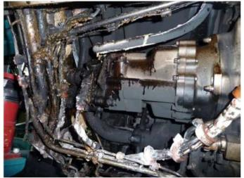
Figure 12: Fire damage to the fuel pump
