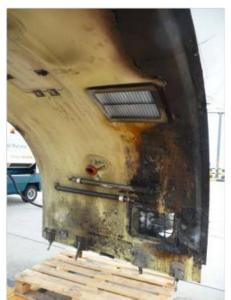
Figure 10: Interior of No.2 engine right fan cowl door
