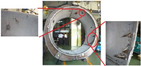
Figure 6: Engine inlet cowl damaged by debris (front view)
