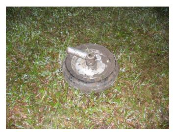
Figure 1. Aircraft nose wheel broken from its axle
