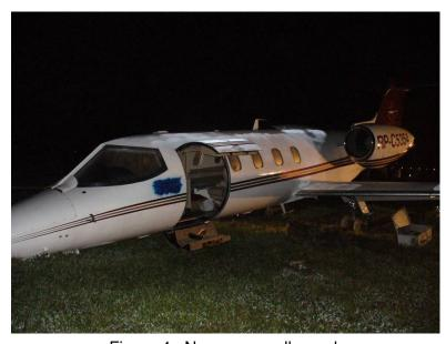
Figure 4. Nose gear collapsed
