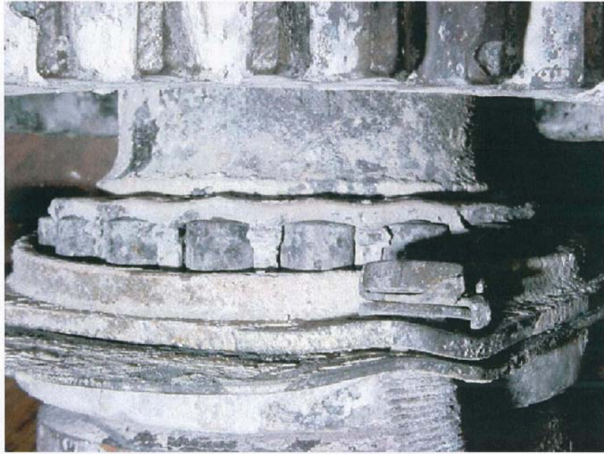
Figure 12: - Forward Starter Drive Bearing Showing the condition of the bearing during engine teardown. Note the cage is deformed at each roller.
