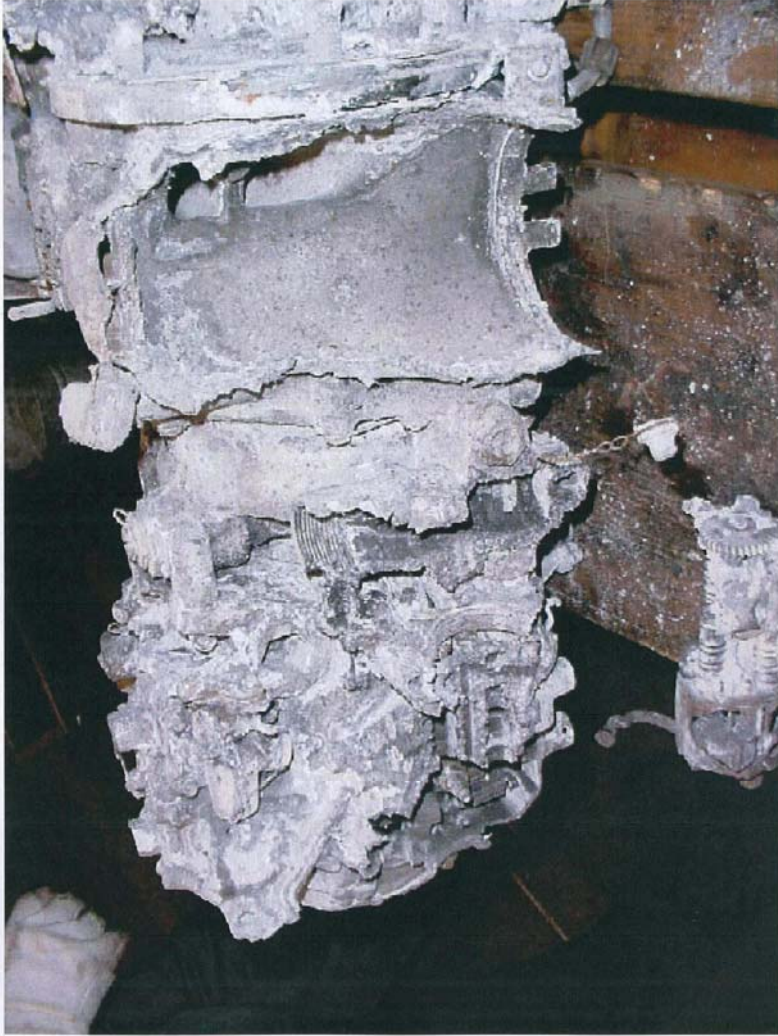
Figure 17: - Fuel Control and Fuel Pump Showing the condition of these units at engine teardown. These housings exhibited numerous areas of localized melting, which had resulted in the severe distress to these units.
