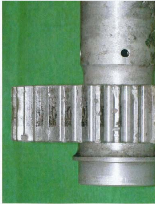
Figure 11: - Starter Drive Gear Showing contact patterns and smeared impact damage along the gear teeth of the starter drive gear.
