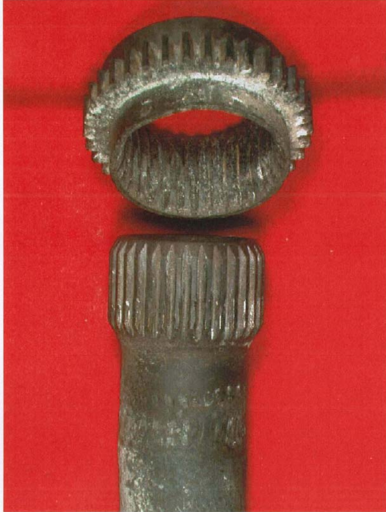
Figure 6 : - Layshaft and Ring-Lock Spline Showing spline impressions on the layshaft indicating it had come out of mesh with the Ring-Lock Spline.
