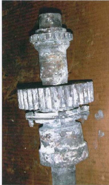
Figure 9 : - Starter Drive Gear Showing the condition of the gear during engine teardown (left) and (right) after disassembly.
