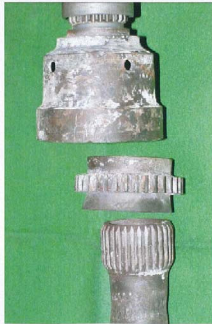
Figure 8 – Ring-Lock Spline Showing the condition of the ring lock spline, which was deformed uniformly around its circumference (shown at right compared to a new spline).
