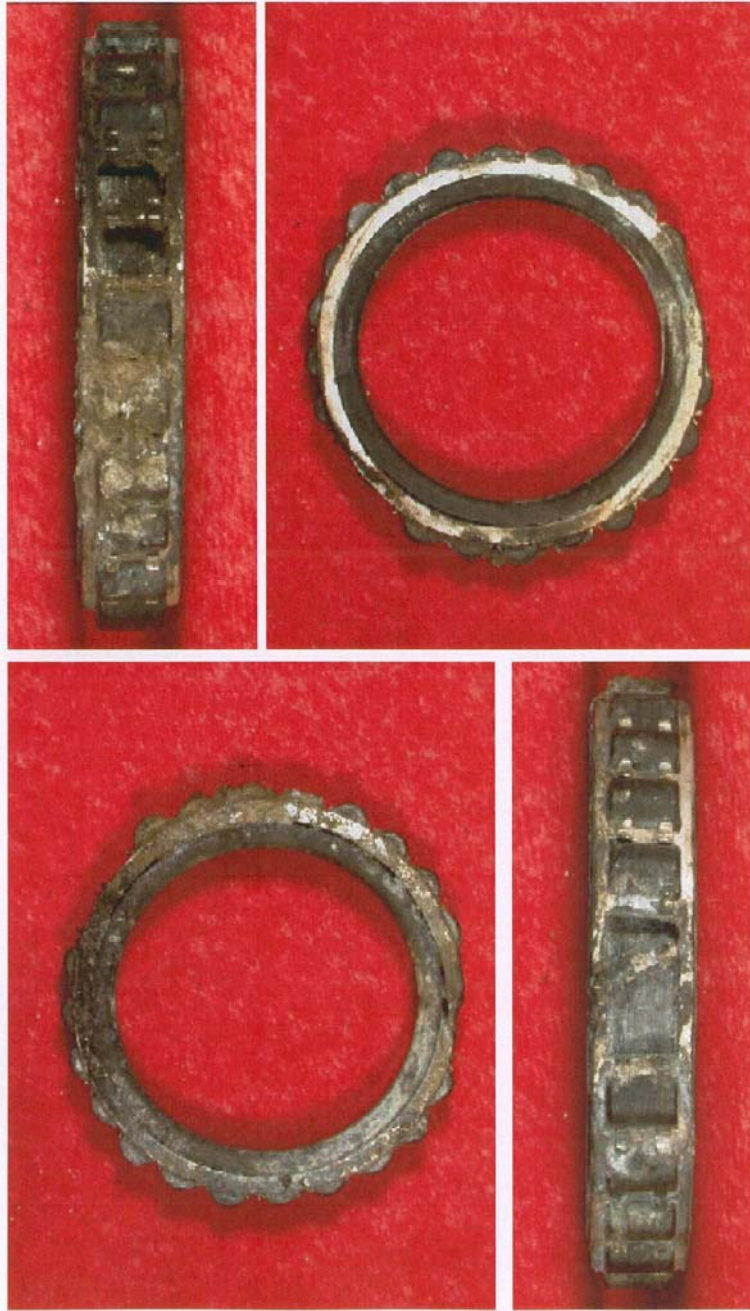
Figure 14: - Rear Starter Drive Bearing Showing the condition of the bearing, which exhibited heavy impact damage.
