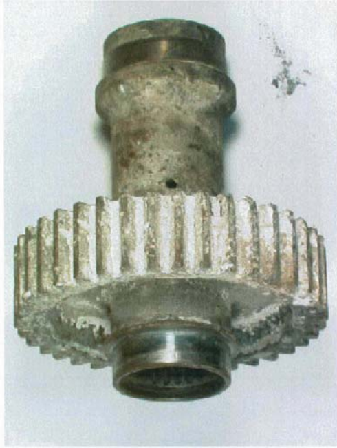
Figure 9 : - Starter Drive Gear Showing the condition of the gear during engine teardown (left) and (right) after disassembly.
