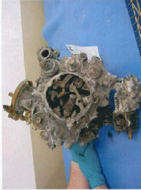
NWA GEARBOX FIRE INCIDENT JFC68-3 SHOWING MAIN COVER DOME MISSING
