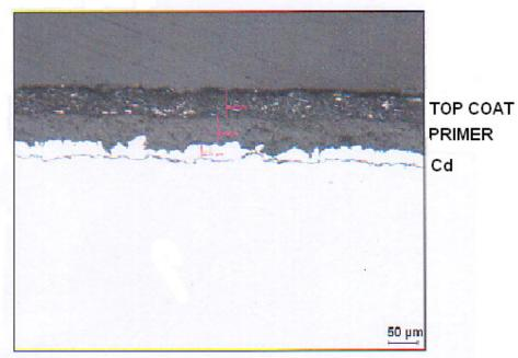
Figure A5: Micrograph showing the top coat, primer and cadmium plating.
