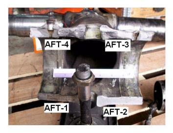
Figure A2: Designation of the aft fractured surfaces
