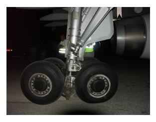
Figure 1: Left hand MLG bogie beam failure
