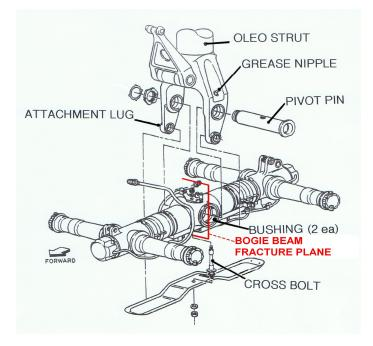
Figure 3: Bogie beam fracture plane
