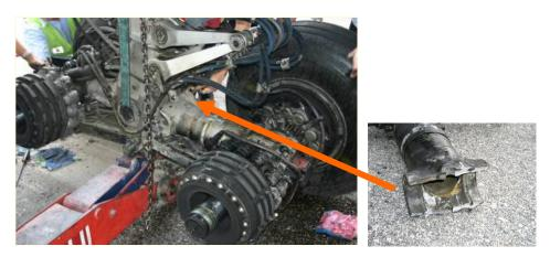
Figure 2: The bogie beam fractured into two parts at the level of the bogie pivot pin attachment hole.
