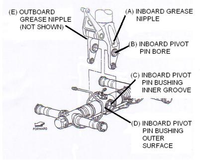
Figure A6: Bogie beam grease sample locations
