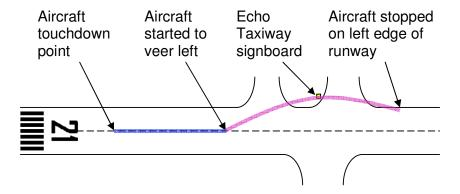
Figure 1: Ground path of the aircraft (Not drawn to scale)
