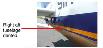
Figure 3: Damage of right aft fuselage
