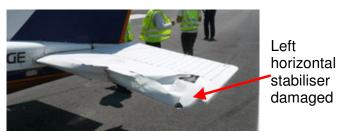
Figure 2: Damage of horizontal stabiliser
