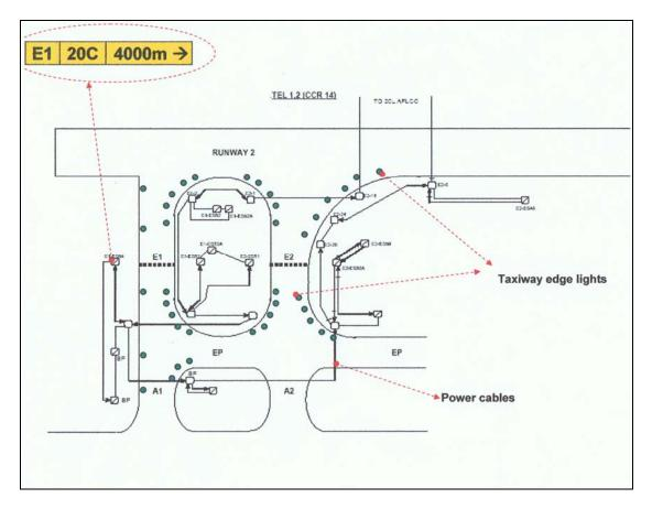
Figure 9. Guidance Signs Control Circuitry
