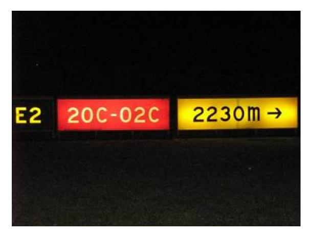
Figure 6. Guidance sign at E2 taxiway holding position after the original inscription panel showing 3850 m was replaced with one showing 2230 m
