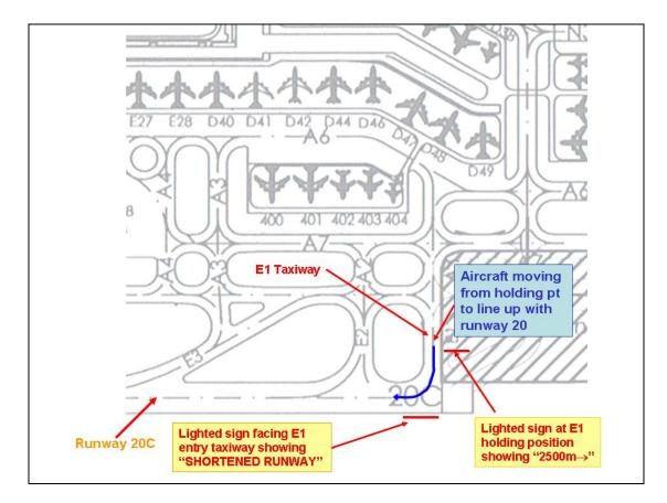
Figure 8. Positions of the guidance signs
