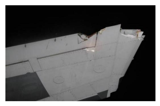
Figure 3. 9V-SVO damage at right wingtip and aileron. View from rear / below.
