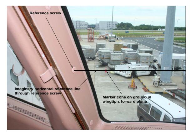
Figure 4 – Side view from pilot's (left) seat, using a screw located on a window frame as a reference to judge wingtip clearance.
