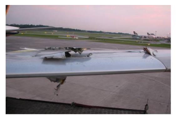
Figure 2. 9V-SVH damage at top of left wingtip area. View from front / above
