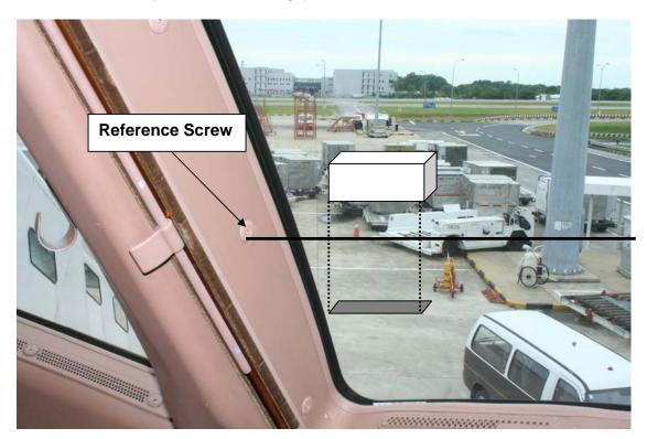
Figure 5 Mid-air object represented by the white box appears to be above reference screw.
