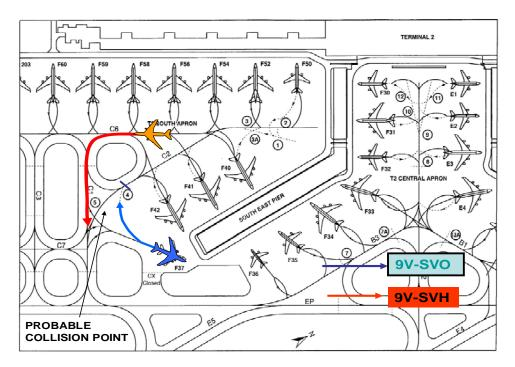
Figure 1. Tracks of 9V-SVH and 9V-SVO, prior to collision.
