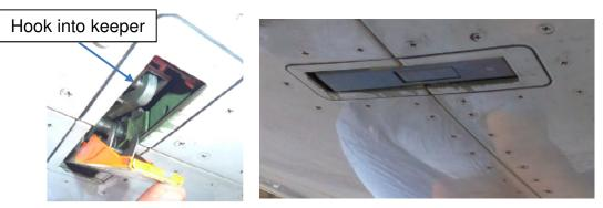
Figure 7: Fastened latch with hook into keeper, and handle closed flush
