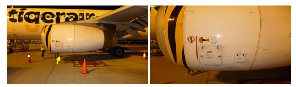
Figure 13: (Left) Unfastened latches can barely be seen from a distance (side of engine) (Right) Unfastened latches cannot be seen when standing next to engine
