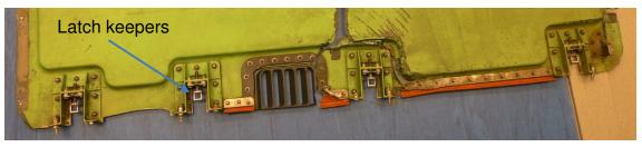
Figure 5: No damage to the hooks and keepers of the latches
