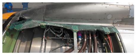
Figure 2: Damage on the engine forward pylon
