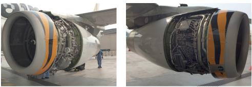
Figure 1: Loss of inboard and outboard fan cowls
