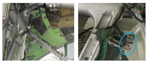
Figure 6: (Left) Fan cowl debris wedged into left main landing gear door (Right) Proximity sensor (blue circle) impacted by fan cowl debris
