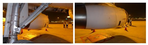
Figure 14: Unfastened latches cannot be seen at any point from the main landing gears to the engine
