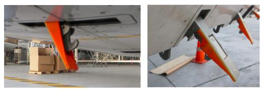
Figure 8: Protrusions due to unfastened latches
