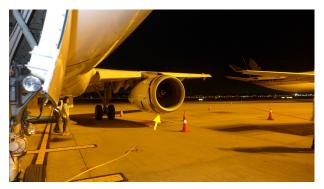
Figure 15: Unfastened latches can barely be seen from the nose landing gear location
