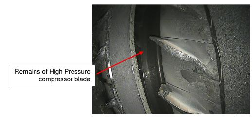
Figure 4: All HP compressor blade aerofoils missing
