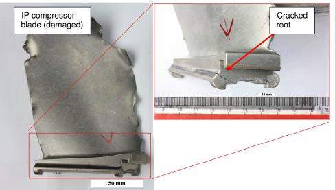
Figure 2: Cracked IP compressor blade root
