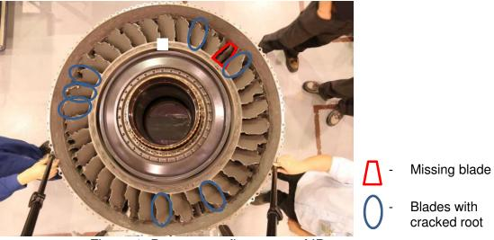
Figure 1: Damage on first stage of IP compressor
