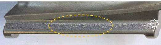
Figure 5: Galling observed at IP compressor blade root
