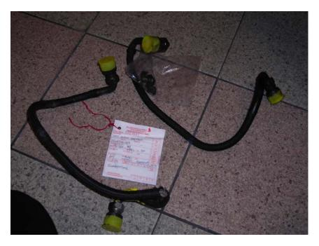
Figure 8: Damaged brake temperature harness
