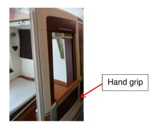
Figure 8: Window frame of Suite Class seat partition
