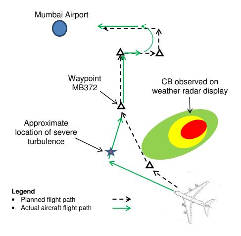
Figure 1: Aircraft flight path (not to scale)
