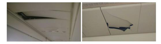
Figure 2: Damaged ceiling panels in cabin
