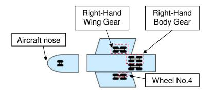
Figure 2: Landing gears of B744F (plan view)
