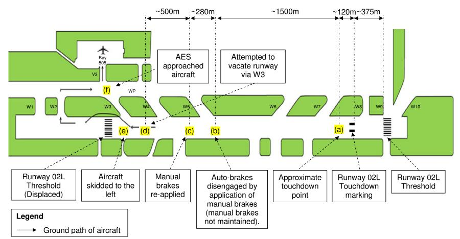
Figure 1: Ground path of the aircraft (Not drawn to scale)
