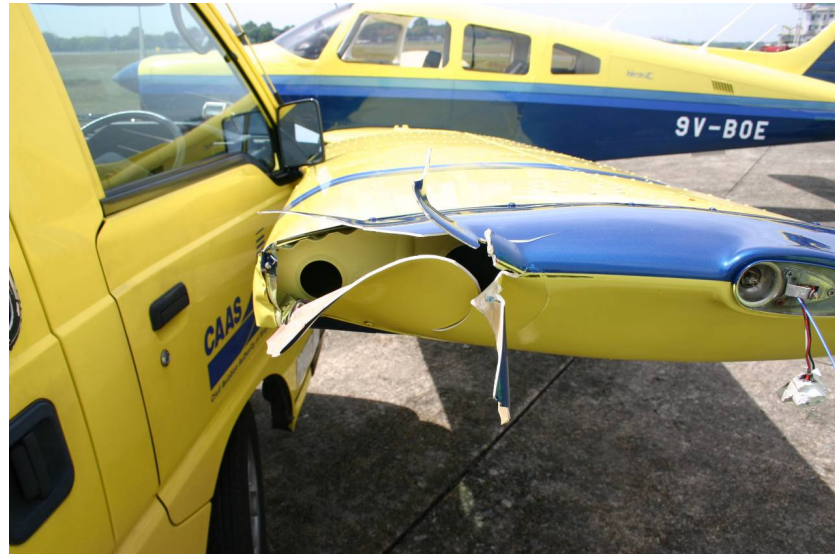
Figure 3. Damage to the aircraft
