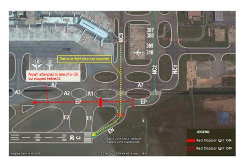
Figure 2: Taxiway centerline lights (in green), ground path of aircraft (in red), and taxi route expected by the flight crew (in yellow).
