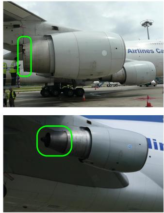
Figure 2. Side view of the damaged No.4 engine (upper picture with missing engine component) and the typical view of an undamaged engine (lower picture)
