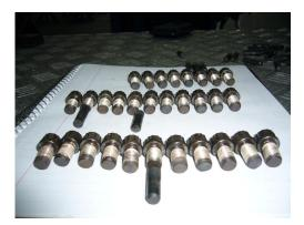
Figure 14. Broken combustor pins exhibiting fatigue wear
