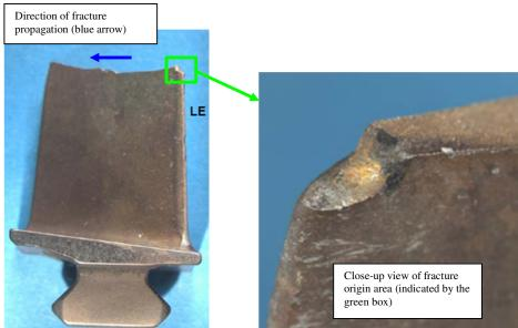
Figure 8. S9 HPC blade showing fracture origin area and direction of fracture propagation (indicated by blue arrow)
