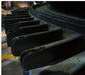
Figure 10. Some of the thirteen S1 high pressure turbine (HPT) blades found damaged with nicks, oxidation or cracks
