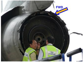
Figure 3. Rear view of the damaged turbine section
