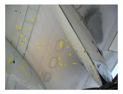
Figure 5. Damage on the No.4 pylon, fuel tank access panel and the lower wing surfaces
