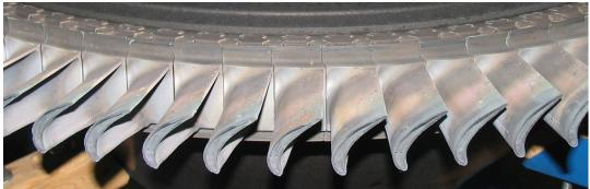
Figure 11. No signs of damage on the rest of the S1 HPT blade
