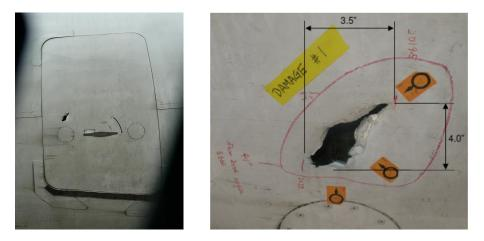
Figure 6. Damage on bulk cargo door
