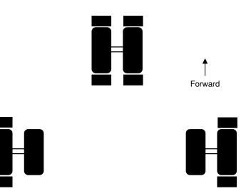
Figure 5: Wheel chock positions as per operator's Quality Assurance Notice
