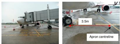
Figure 2: Resting position of the aircraft
