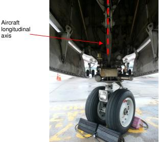
Figure 3: Rotation of NLG wheel (viewed from nose towards aft)
