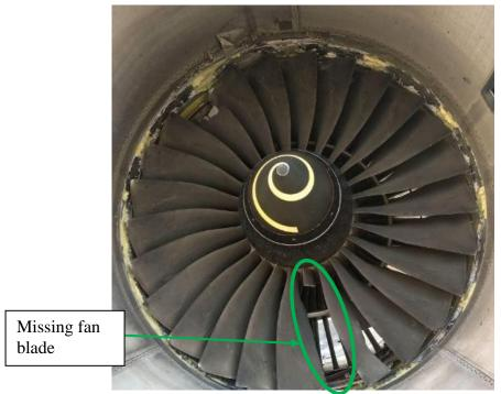
Figure 2: The missing fan blade (circled in green) with more than 75% missing material
