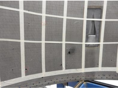
Figure 8: Impact damages on the inner barrel of inlet cowl
