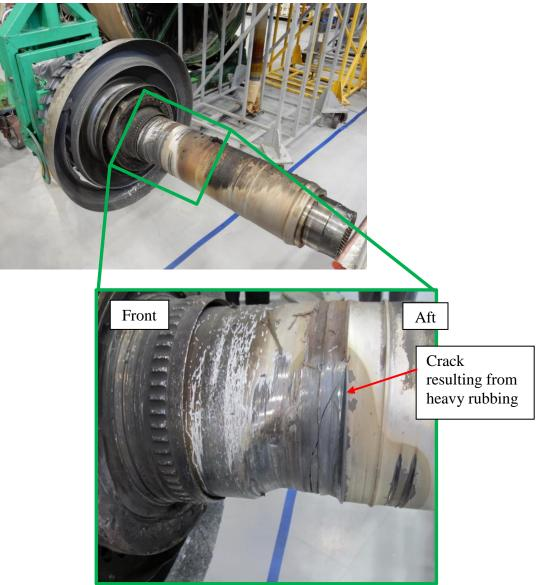
Figure 3: Crack seen on heavily rubbed LP shaft
