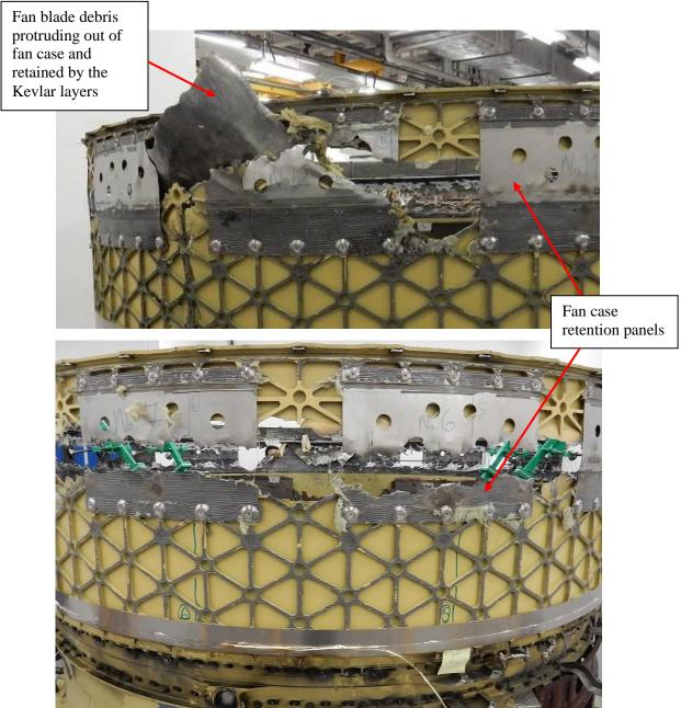
Figure 6: Exterior view of damaged fan case (with Kevlar layers removed)
