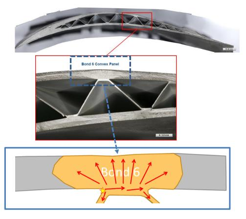
Figure 10: Fatigue failure location (Bond 6) and failure mechanism
