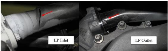
Figure 7: Fractured LP fuel pump inlet and outlet pipes (indicated by red arrows)
