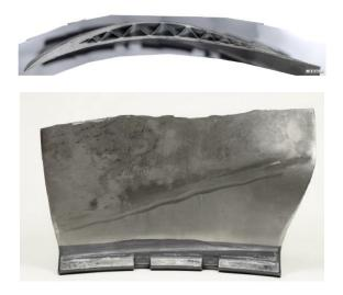
Figure 9: Fan blade segment recovered (side and top view)
