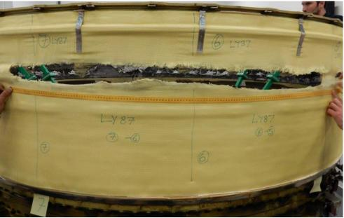
Figure 5: Damaged Kevlar layers (viewed from exterior)
