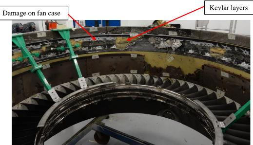
Figure 4: Damage on the fan case (viewed from interior)
