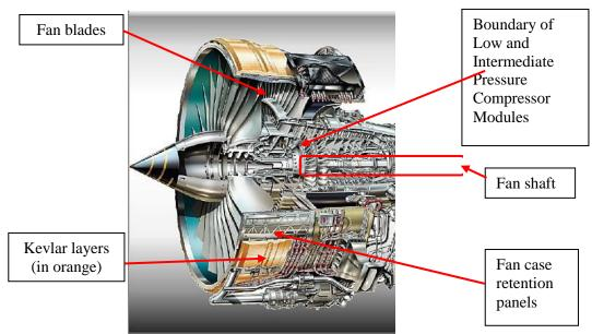
Figure 1: Cutaway view of Trent 700 engine fan case
