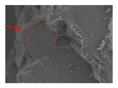
Figure 11: Fatigue failure initiation site in the membrane material adjacent to the diffusion bond (region indicated in red).
