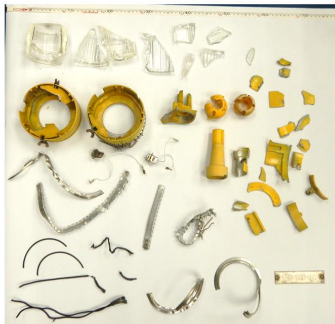
Figure 5: Debris from the broken runway edge lights
