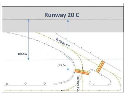
Figure 7. Distance from Runway 20C centreline to E6 runway holding position marking
