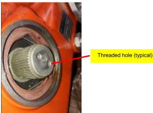
Figure 15: Output shaft of the engine gear box (output flange removed for clarity)
