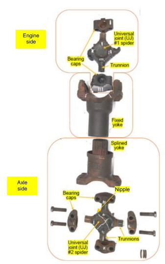
Figure 7: Tranmission shaft assembly
