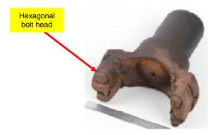
Figure 19: Hexagonal bolt heads on the fixed yoke of the cleaned-up transmission shaft assembly
