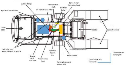
Figure 6: Tow tug schematic
