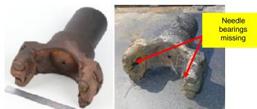
Figure 13: Fixed yoke segment of the transmission shaft assembly (left photo showing the component after cleaned-up)
