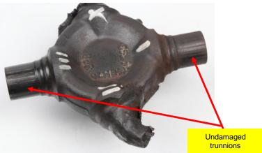
Figure 17: Undamaged trunnions
