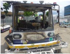
Figure 3: Damage to the driver's cabin of the tow tug
