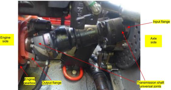
Figure 8: Transmission shaft assembly in situ
