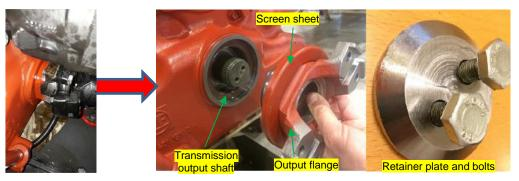
Figure 9: Retainer plate holding output flange (illustration picture only)
