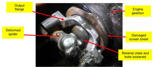
Figure 16: Deformed spider of universal joint
