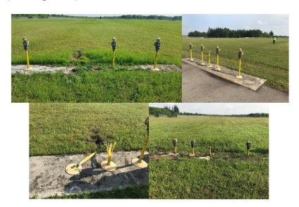
Figure 1. Damaged approach lights
