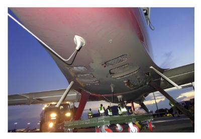
Figure 5: Heat damage on the lower fuselage of aircraft
