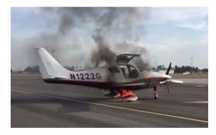
Figure 3: Fire at the main landing gears of the aircraft
