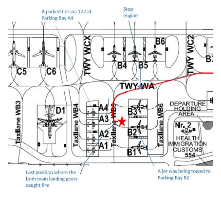
the middle of Taxilane WB5 and facing parking bay B2 (see Figure 2), with the nose gear at  $60^{\circ}$  to the left.
