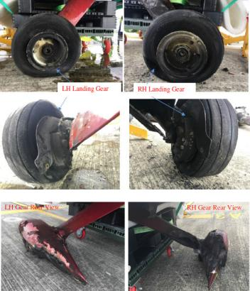
Figure 4: Damage to the landing gears
