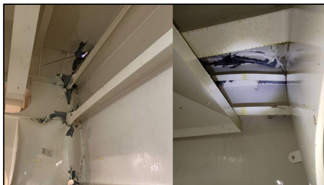
Figure 19 – Deformed shell plating between frames 45 and 52 on port side cylinder oil storage tank ( Source: EB )
