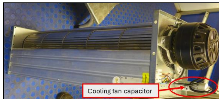
Figure 12 – Sample of the cooling fan capacitor shown by the Electrician (Source: the TSIB)
