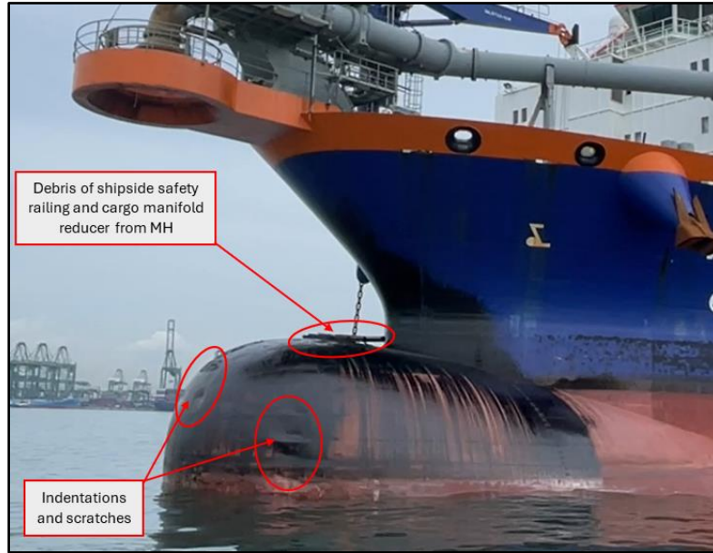
Figure 14 – View of VM's bulbous bow with damages and debris from MH (Source: the TSIB)
