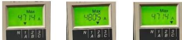
Fig 2 : Max Current at L1, L2, L3 of AFT PS ACB
