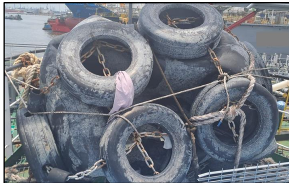
Figure 16 – Yokohama fender (same type as the sunken ones) (Source: MH-Company, from another bunker tanker)
