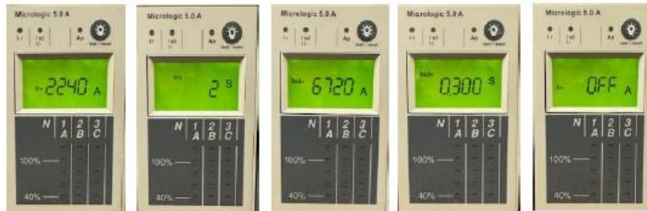
Fig 3 : Protection setting of Micrologic 5.0A at Bus Tie
