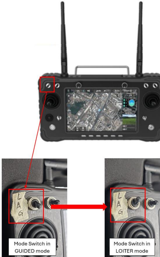
Figure 5: UA RC Mode Switch in three positions: “G” (GUIDED mode), “A” (ALT_HOLD mode) and “L” (LOITER mode)
