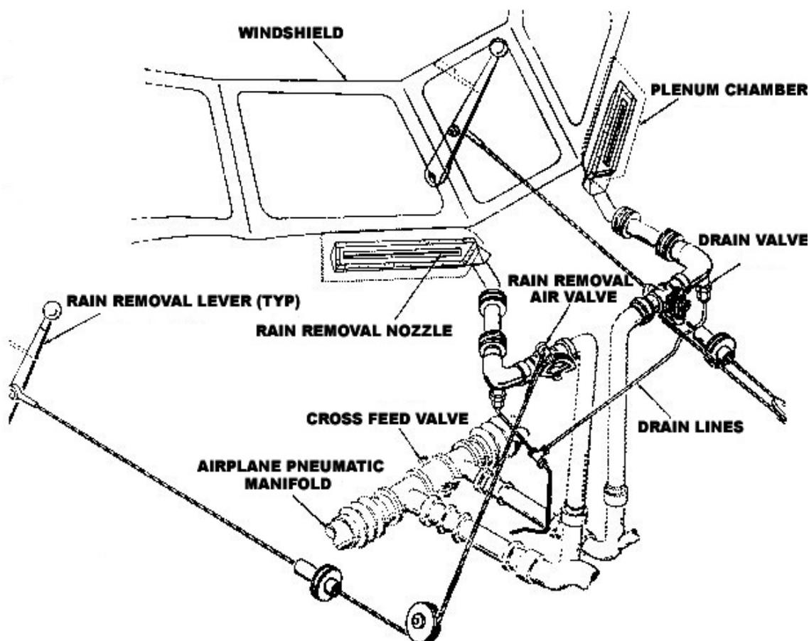
Figure 1. Windshield rain removal system
