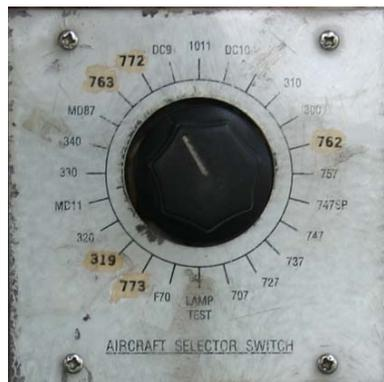
Figure 7. RLG types B and C aircraft type selector knob
