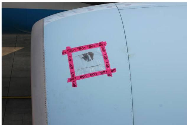
Figure 1. Left engine cowling damage location at 1 o'clock position
