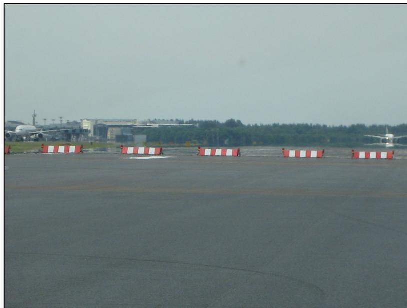
FIGURE 2 – A typical row of marker boards and lights, as placed at 260 m from the temporary runway end lights
