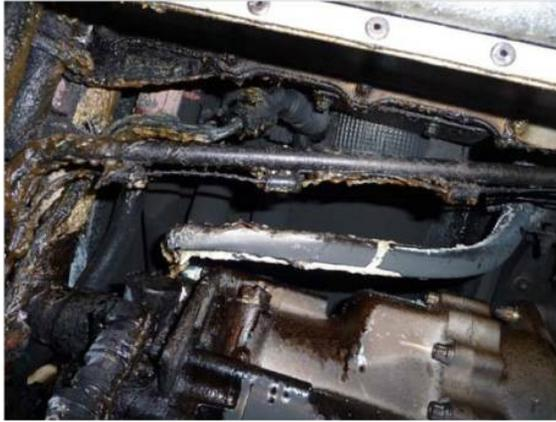
Figure 11: Fire damage to the AOHE
