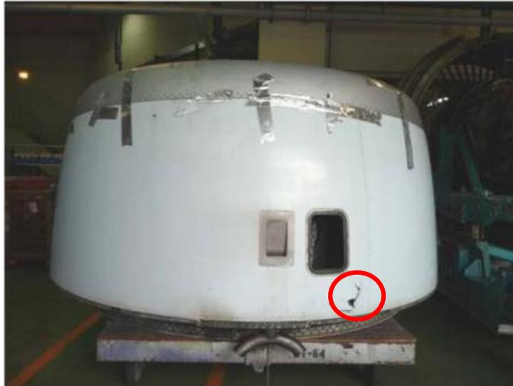
Figure 7: Puncture on engine inlet cowl outer skin (top view)
