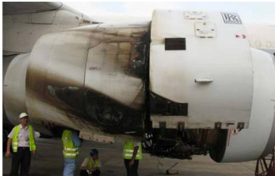
Figure 9: Right side of No.2 engine
