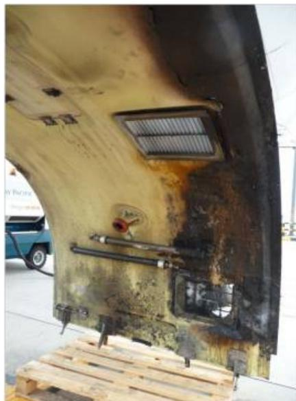
Figure 10: Interior of No.2 engine right fan cowl door
