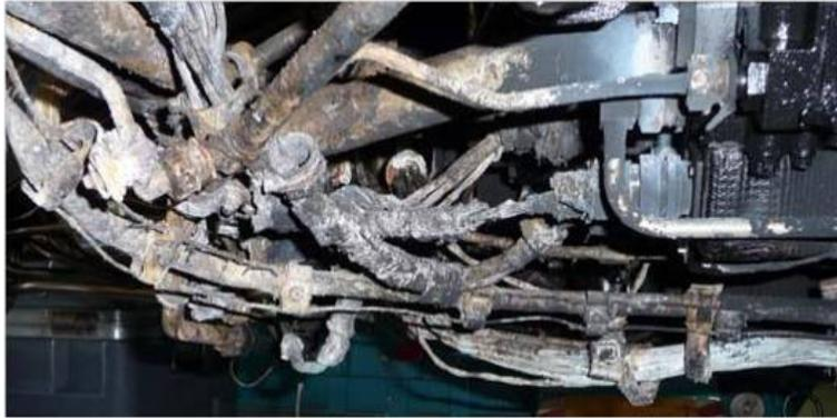
Figure 14: Fire damage to underside of fan case
