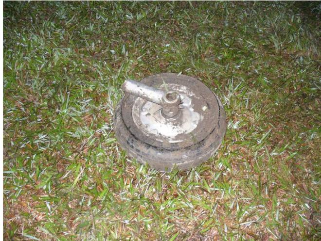
Figure 1. Aircraft nose wheel broken from its axle
