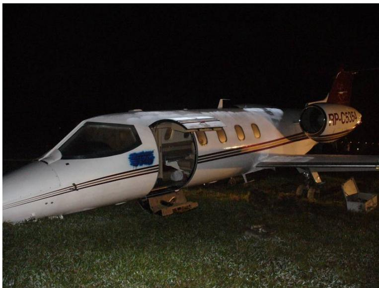
Figure 4. Nose gear collapsed
