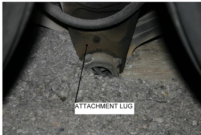
Figure 4: The left MLG oleo strut attachment lugs dug into the asphalt
