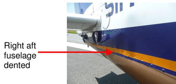
Figure 3: Damage of right aft fuselage
