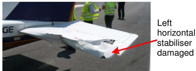
Figure 2: Damage of horizontal stabiliser
