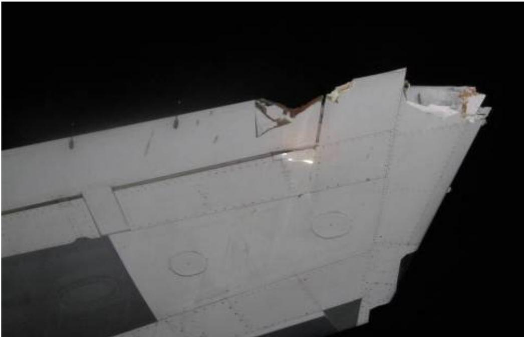
Figure 3. 9V-SVO damage at right wingtip and aileron. View from rear / below.
