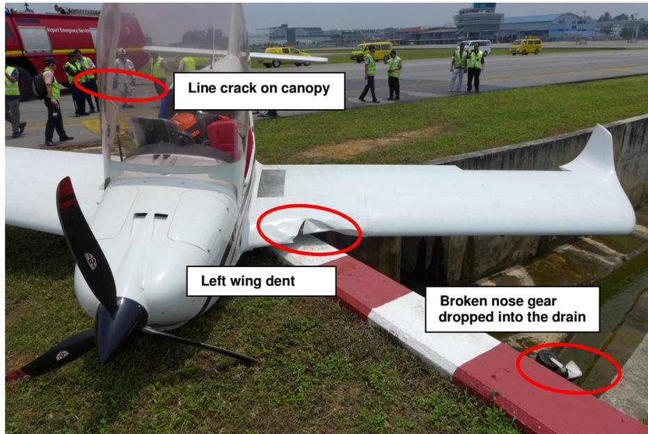
Figure 3: Damage to the aircraft
