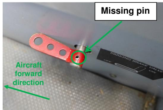
Figure 7: Close up view of parking brake lever
