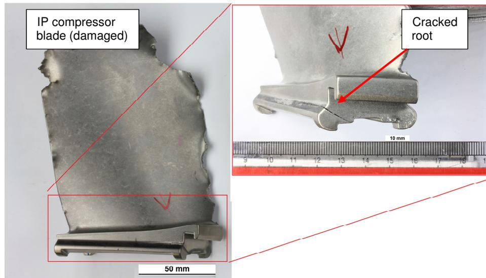
Figure 2: Cracked IP compressor blade root
