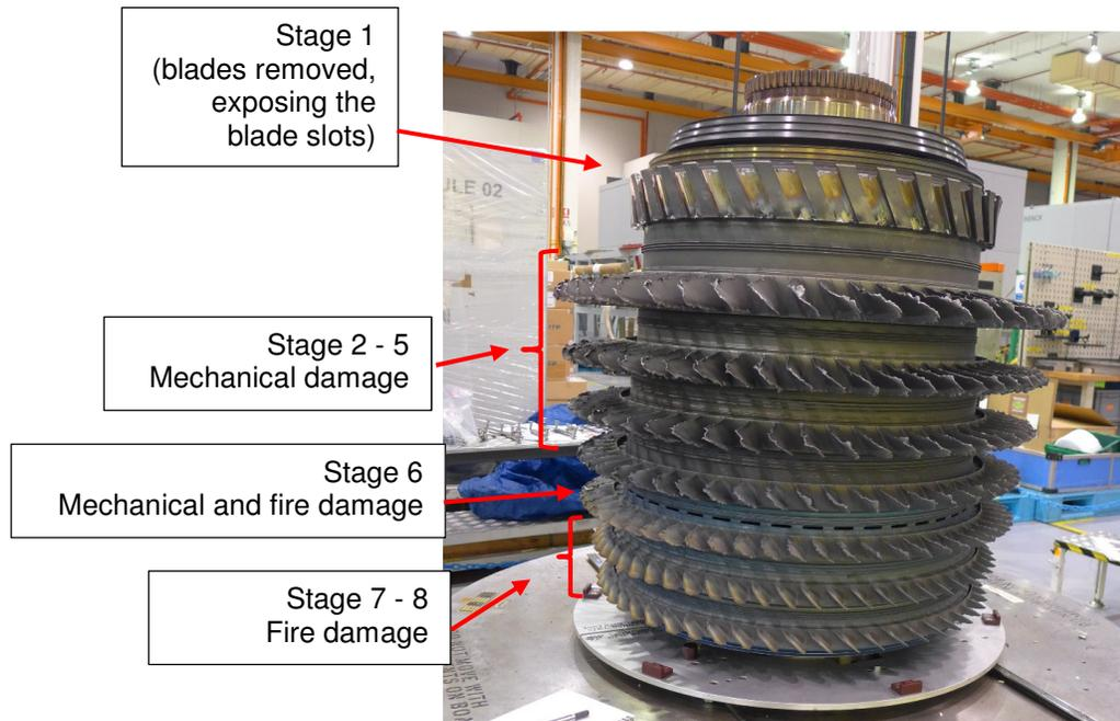
Figure 3: Damage to IP compressor blade aerofoils
