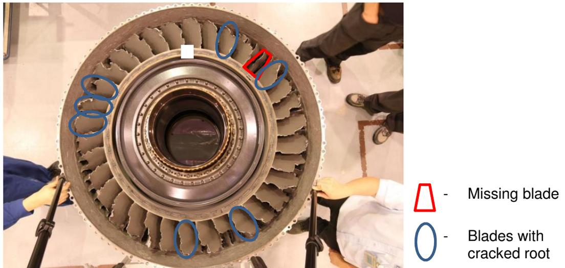
Figure 1: Damage on first stage of IP compressor
