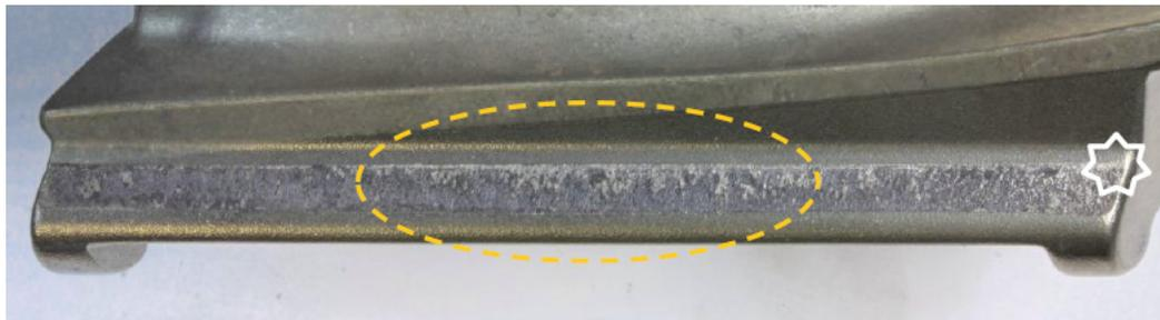
Figure 5: Galling observed at IP compressor blade root
