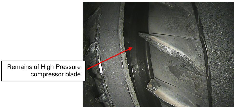
Figure 4: All HP compressor blade aerofoils missing
