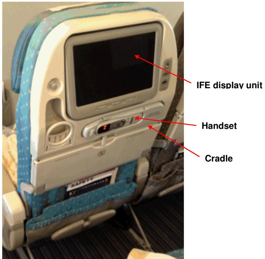
Figure 2: IFE components at each passenger seat
