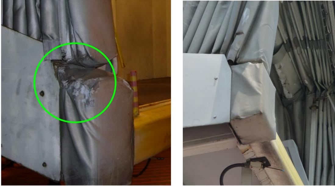
Figure 5: (Left) Damaged padding on incident PLB
