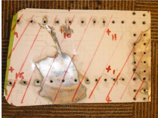
Figure 15: Cut out of the damaged aircraft skin
