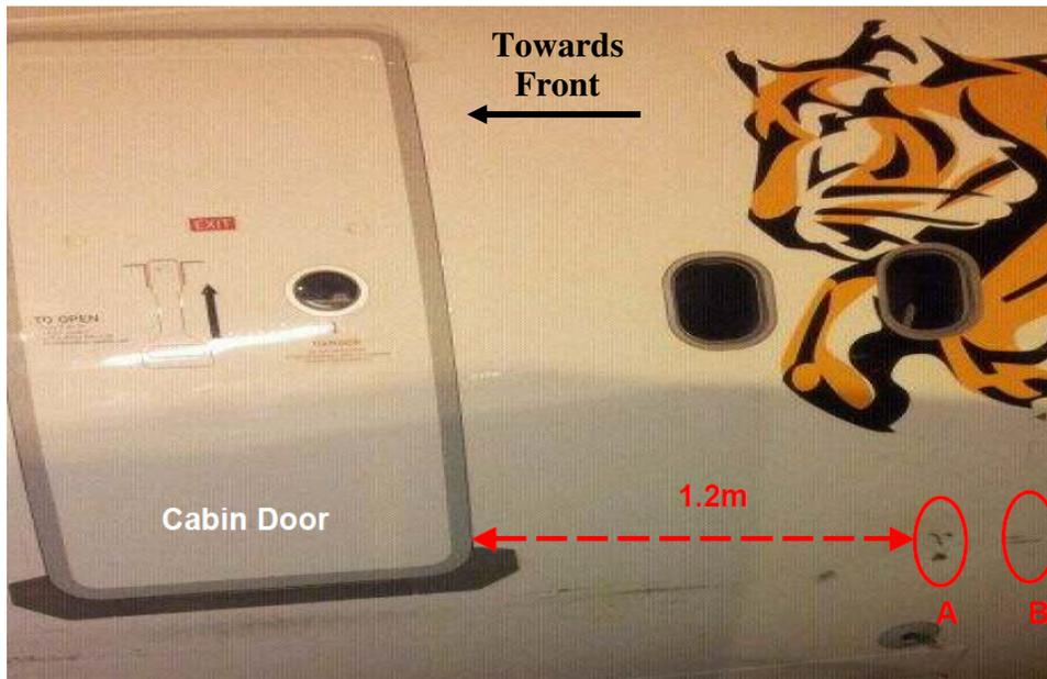
Figure 1: Location of damage on aircraft fuselage
