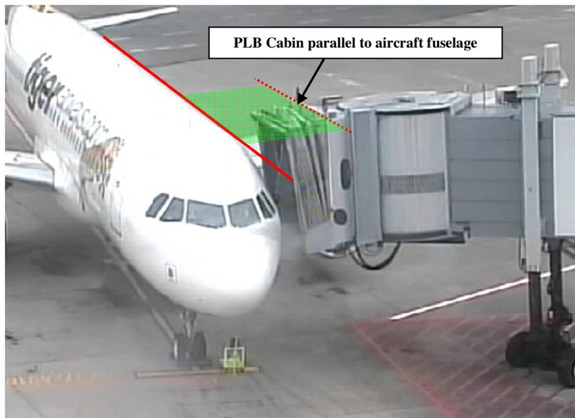
Figure 9: Docking position of PLB on first receipt of aircraft at Bay E7
