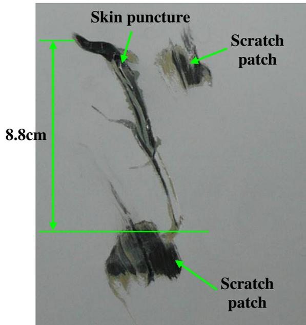
Figure 2: Close-up of damage area A
