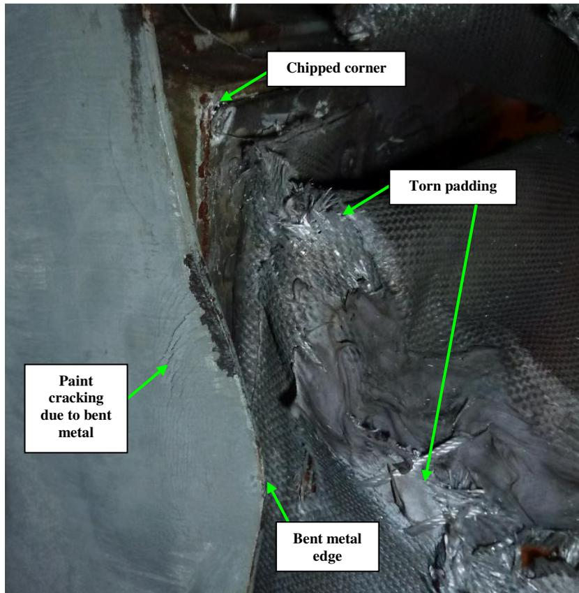
Figure 6: Details of the damaged padding of PLB
