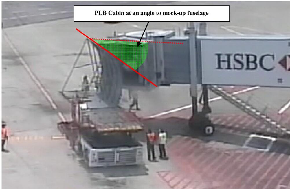
Figure 11: Non-parallel docking position of PLB during simulation
