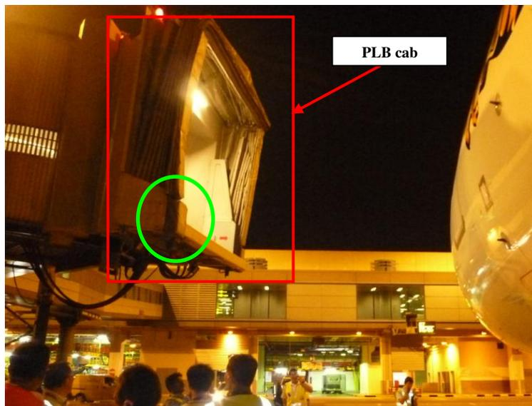
Figure 4: Damage area (green circle) on PLB cab
