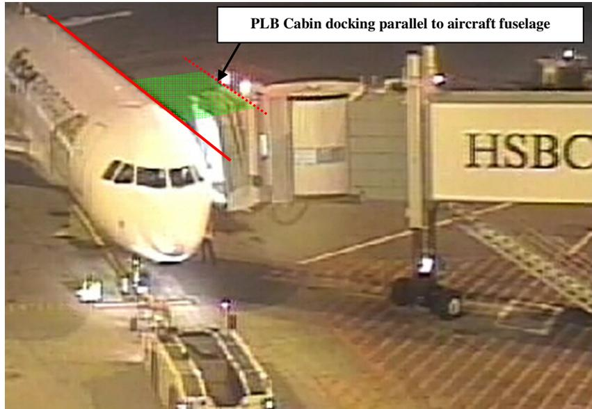
Figure 8: Docking position of PLB after occurrence (performed by another operator)
