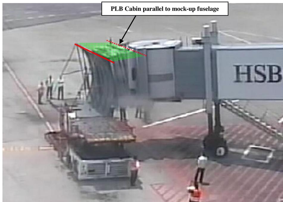
Figure 10: Normal docking position of PLB during simulation
