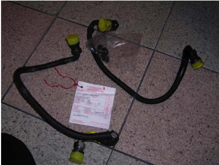
Figure 8: Damaged brake temperature harness
