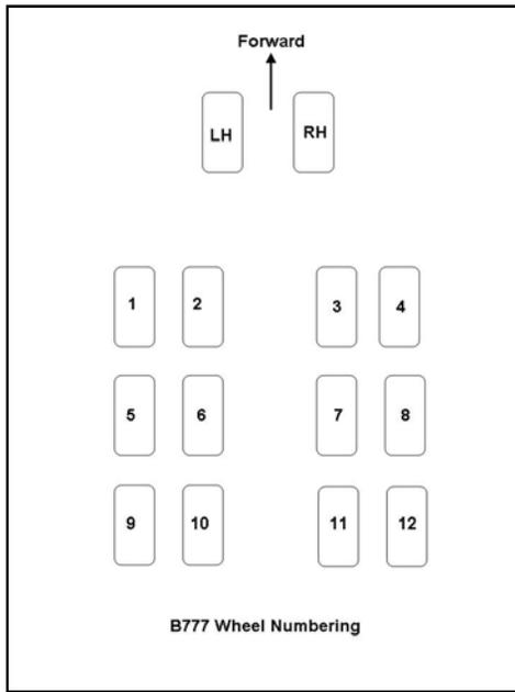
Figure 5: B777 wheel numbering system
