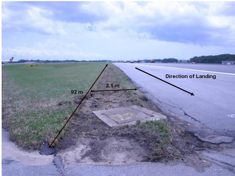
Figure 3: Wheel track on grass patch adjacent to runway edge (looking against the direction of landing)
