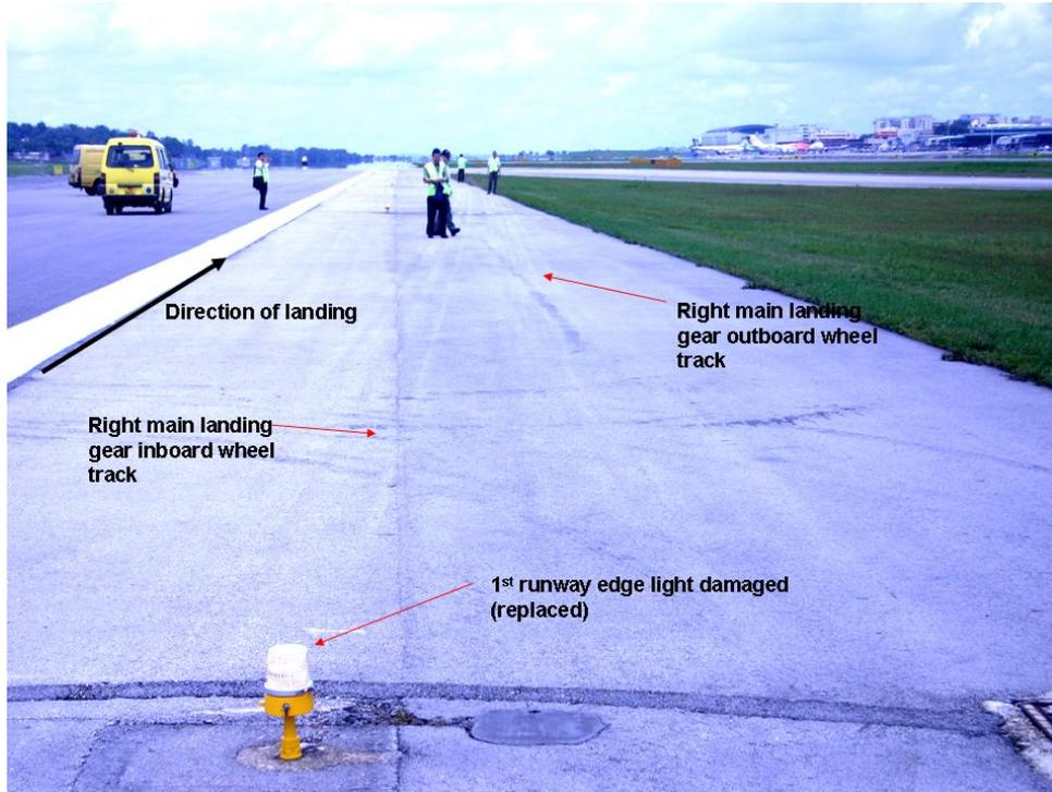
Figure 2: Wheel track of right main landing gear (looking in the direction of landing)
