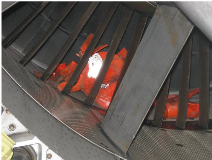
Figure 1: Cone ingested into the No. 2 engine
