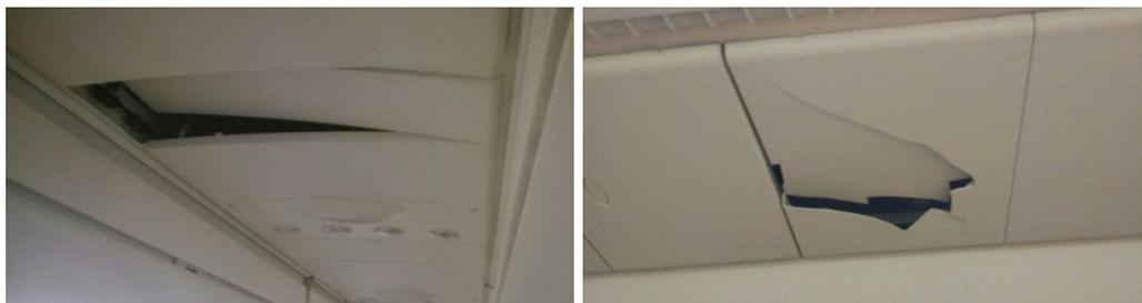
Figure 2: Damaged ceiling panels in cabin
