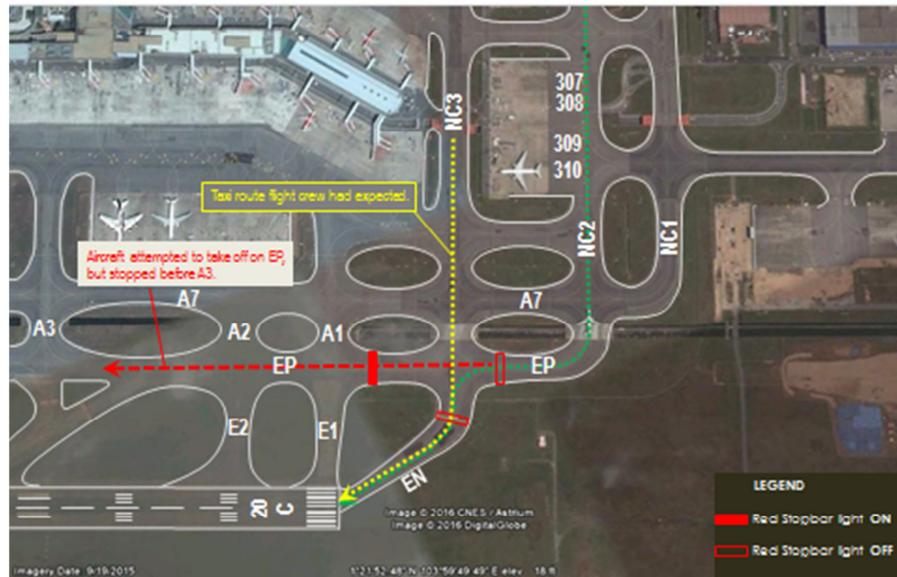
Figure 2: Taxiway centerline lights (in green), ground path of aircraft (in red), and taxi route expected by the flight crew (in yellow).
