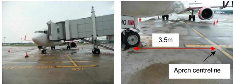
Figure 2: Resting position of the aircraft
