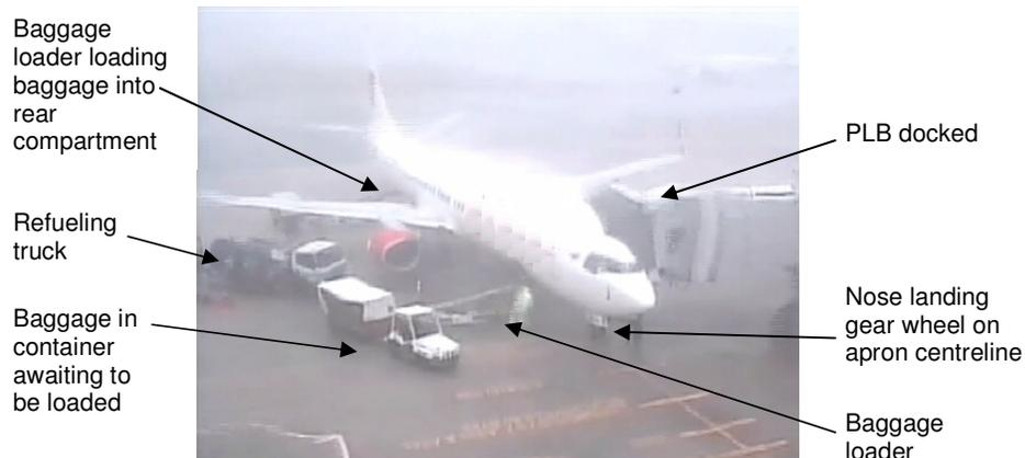
Figure 1: Positions of aircraft, PLB, baggage loader and refueling truck
