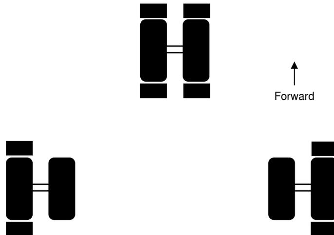
Figure 5: Wheel chock positions as per operator's Quality Assurance Notice
