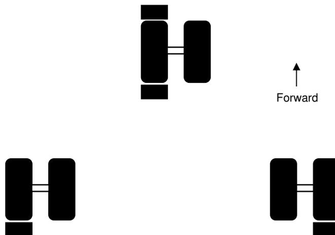
Figure 4: Actual wheel chock positions on incident aircraft
