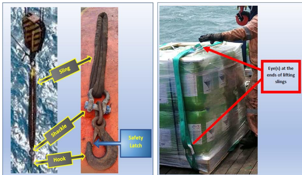
Figure 7: Lifting equipment arrangement of FLC. The lifting sling used by OPL 66 (right) for pallet and IBC tanks. The image (on the right) is for reference only and does not indicate the pallets in use at the time of occurrence – annotated by TSIB.
