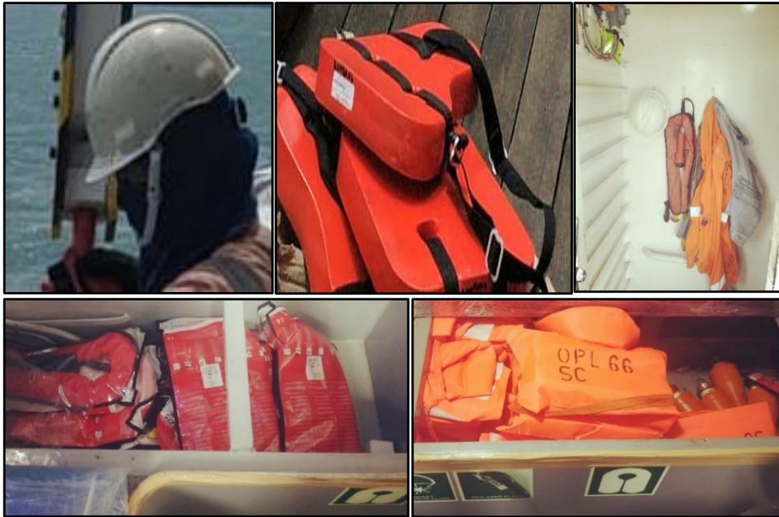
Figure 6: (Clockwise from top left) Helmet with chinstrap, work life-vests used on the boats, the PPEs - inflatable lifejacket and clothing of the deceased (engineer) hanging at the engine room access (post incident), SOLAS lifejackets as per the LSA plan and additional inflatable lifejackets for passenger transfers under the passenger benches of OPL 66 Source – the Operator
