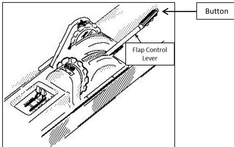
Figure 1. Flap control lever
