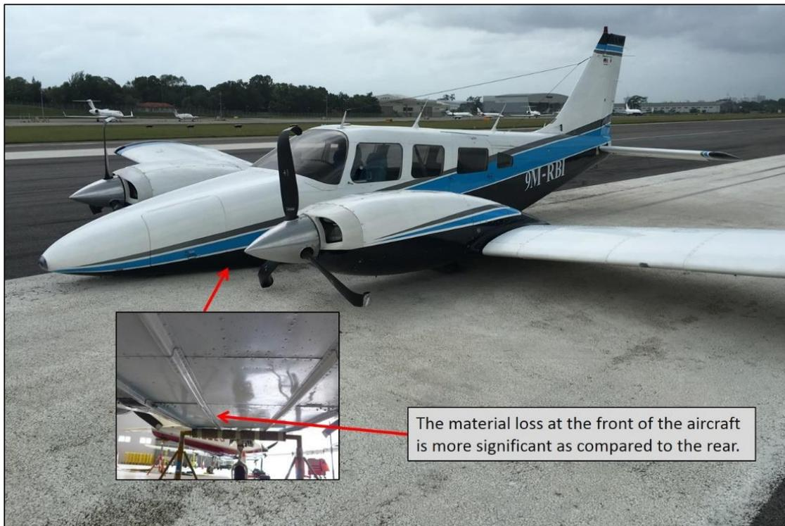
Figure 4. Damage at the belly of the aircraft
