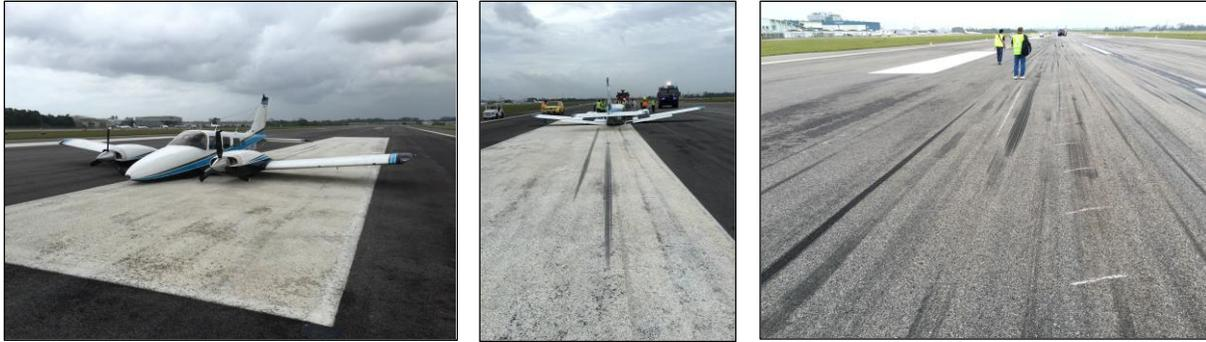
Figure 6. Position of the aircraft and impact marks
