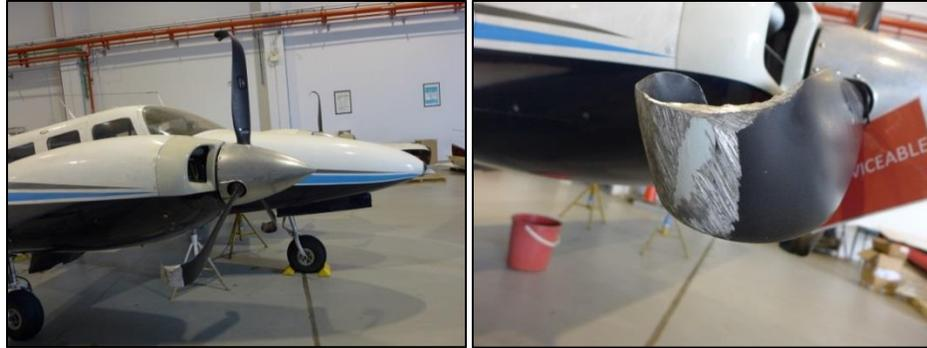
Figure 3. Propeller tip bent forward
