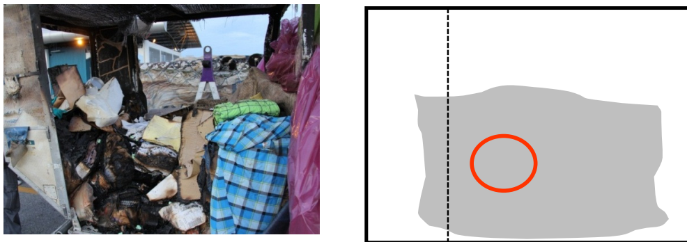
Figure 2: (Left) Cargo container 42L and its contents (Right) Top view of container, red circle denotes area believed to be the fire origin
