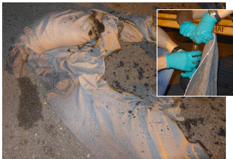
Figure 3: The bale of fabric heavily soaked in alcohol-like fluid. (Inset: Fluid being collected by squeezing the sample of fabric)
