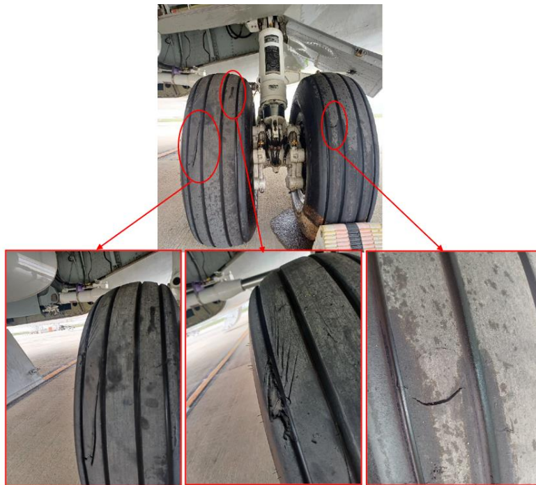
Figure 7: Damages to the right MLG tyres (viewed from the front)
