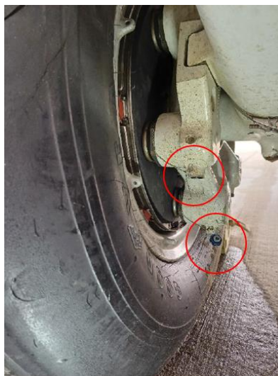
Figure 8: Sheared bleeder plugs of the right MLG outboard brake assembly
