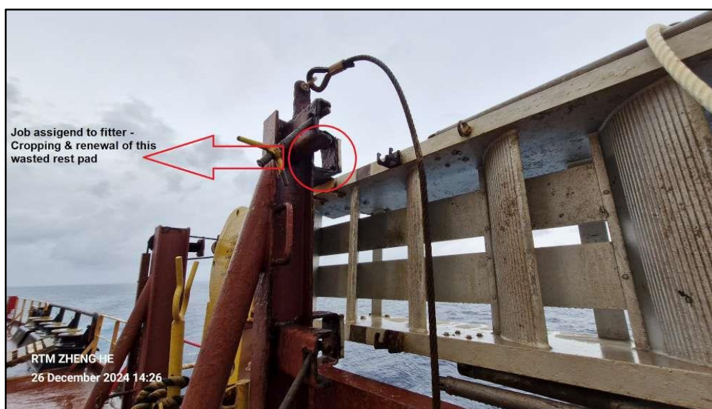
Figure 2 – Location of the rest pads at the port side gangway with annotation (Source: the Company)
